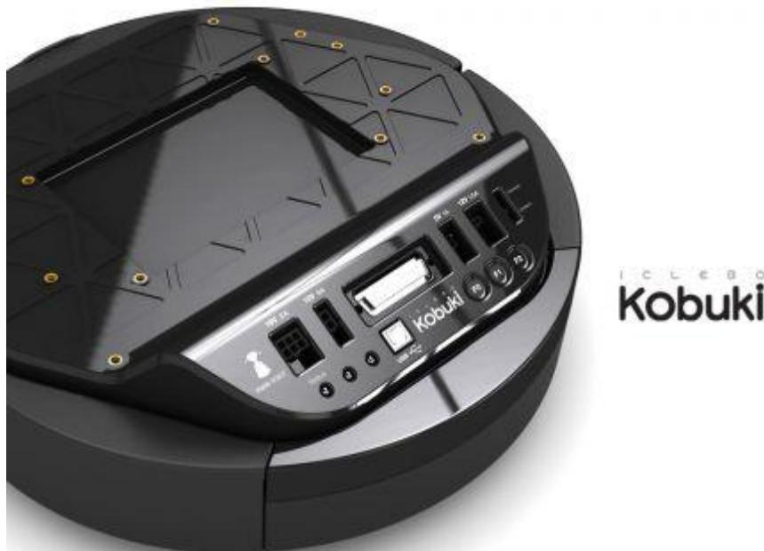
iClebo Kobuki is a low-cost mobile research base designed for education and research on state of art robotics. With continuous operation in mind, Kobuki provides power supplies for an external computer as well as additional sensors and actuators. Its highly accurate odometry, amended by our factory calibrated gyroscope, enables precise navigation.
