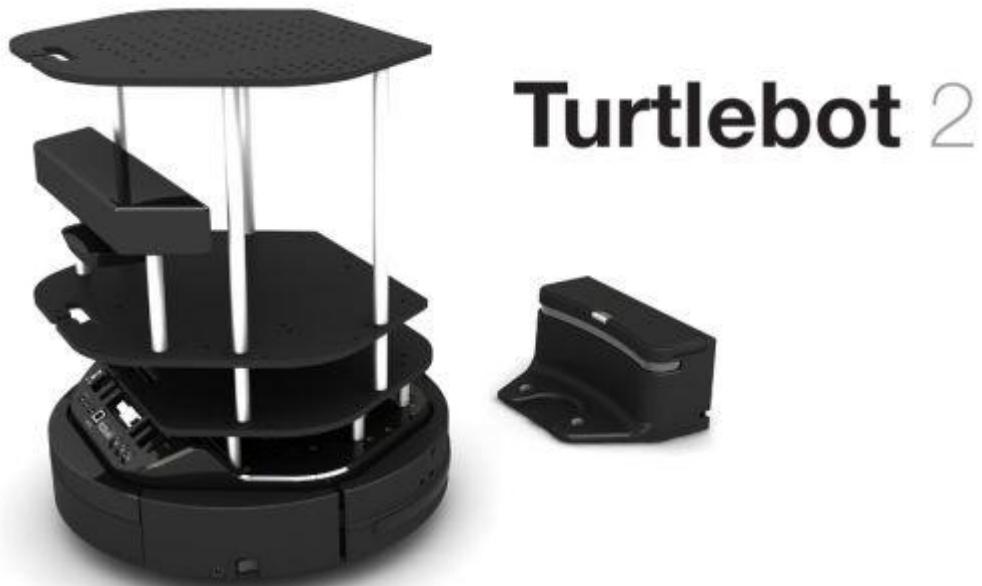
TurtleBot2 is an open robotics platform designed for education and research on state of art robotics. It is also a powerful tool to teach and learn ROS(Robot Operating System) and make the most of this cutting edge technology. Equipped with a 3D sensor, it can map and navigate indoor environments. The 3D perception, together with the turtlebot arm, enables manipulation tasks.
